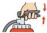
③ Strongly squeeze the handles together to discharge the extinguishing agent inside.
