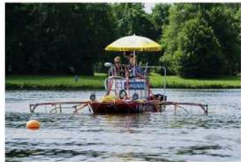
The 'water harrow', the device that was used to bring hydrogen peroxide into Lake Koeshuis.
