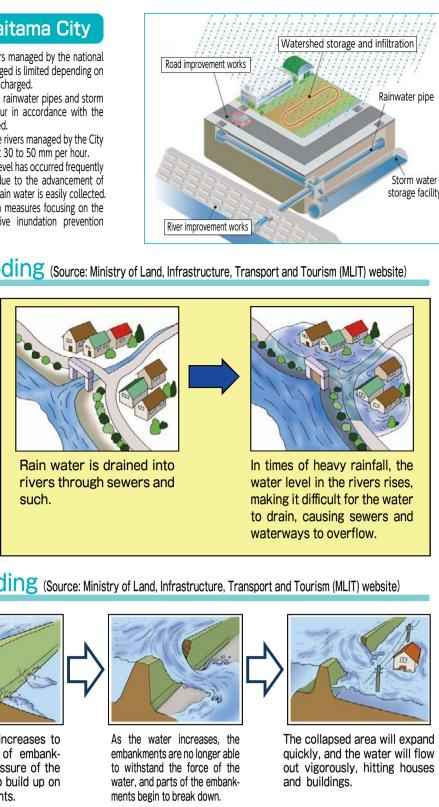
When rainfall exceeds the drainage capacity of sewers, water overflows from sewers or the water which cannot enter sewers remains on the ground.
